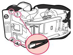
5. Pull elastic loop on the seat pad through the vehicle belt guide on side of seat and attach to hook as shown **3**. Repeat on other side.
